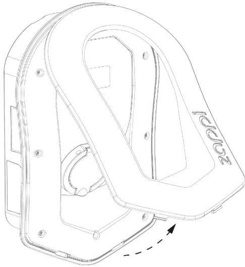
Carefully remove fascia from the zappi by pressing the 2 clips located at the bottom of unit inwards whilst pulling the fascia towards you.
